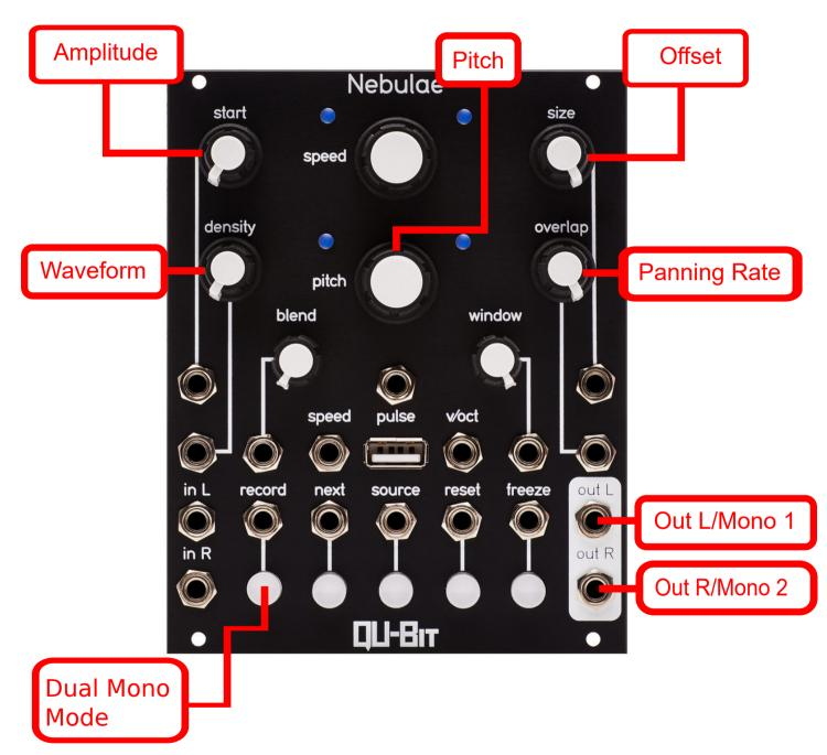
Nine oscillators tuned to very small offsets relative to the main pitch create an effect called "Risset's harmonic arpeggio". Pitch, arpeggiation offset and amplitude controls; six waveforms with morphing; stereo mode has optional cross-panning with speed control; optional dual mono mode (Mono 1: Risset arpeggio; Mono 2: waveform oscillator).
