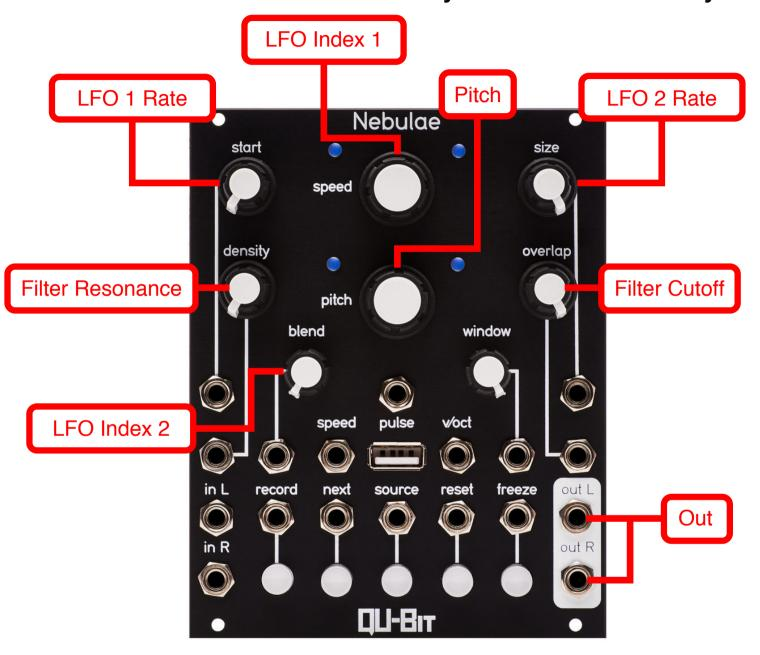
This instrument is a wavetable oscillator that scans three dimensional surfaces. It includes a low pass filter for additional control. Ported from Neb v.1 by Chris Erin.
