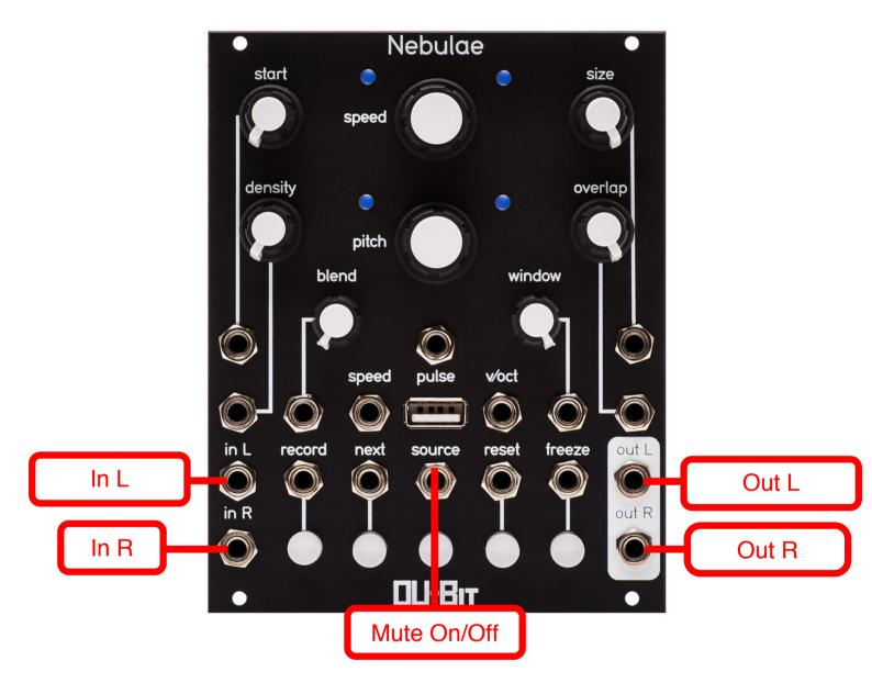
This instrument is a simple template for testing audio input and output, with an added mute button, to test passing an audio signal through the Nebulae. This instrument file can also be modified to process the incoming audio signal with Csound. Simply change the code of the text file and add in as many FX loops and chains as you want. The buttons can be configured for different latching behaviors and the knobs can be set to control the parameters of your new synth instrument.
