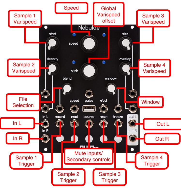
This instrument allows simultaneous playback of four samples at a time. Each sample has it's own pitch control and trigger input. Blend is the offset for file selection: when fully CCW the first four samples loaded on the Nebulae will be played, when fully CW the last four samples will be played.
