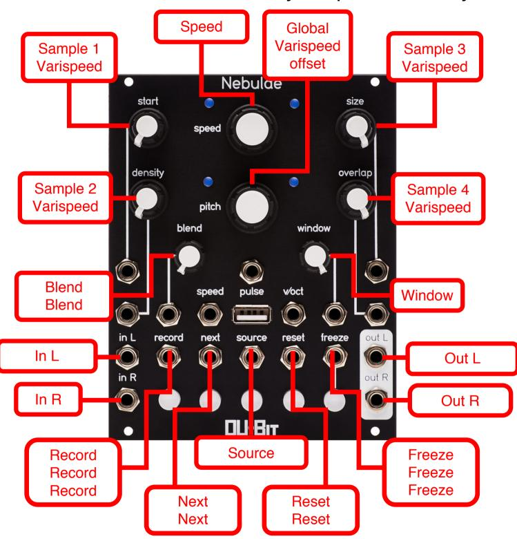
This instrument allows simultaneous playback of four samples at a time. Each sample has it's own pitch control and trigger input.
