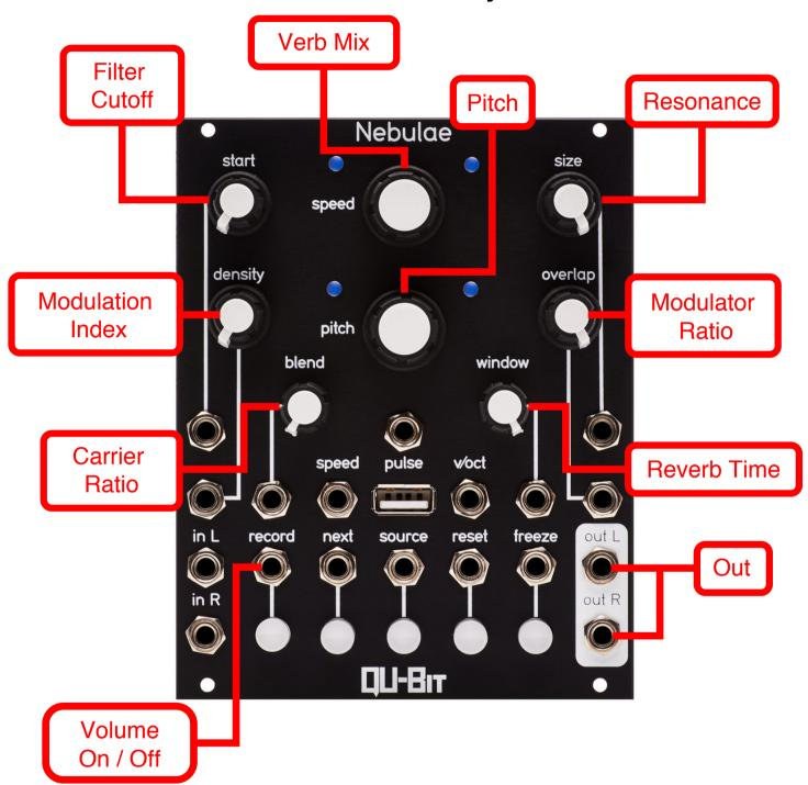
This instrument is an FM synth that generates gritty waveforms with its extreme C:M ratio and modulation index range controls. The resulting signal passes through a Moog-style ladder filter that can optionally be mixed in with Reverb at the output. The volume can also be muted by pressing the "record" button. Ported from Neb v.1 by Chris Erin.
