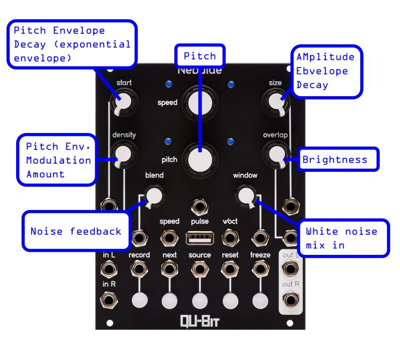
The snare drum is a clocked noise source being fed into a filter. The feedback knob sends the output of the noise sample and hold into the clock frequency over the first half of the knob and into the filter cutoff frequency over the second half. Pure white noise can be fed in with the window knob.
