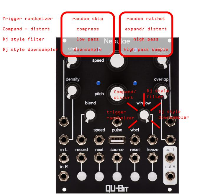
All of the drums have one global effect that is controlled by the 'speed' knob. There are four effects which can be selected between by pressing the source button and turning the window knob. All four effects do something different when the speed knob is left of center versus right of center, indicated by the two LEDs next to the speed knob. The durm program boots with the trigger randomizer by default.
