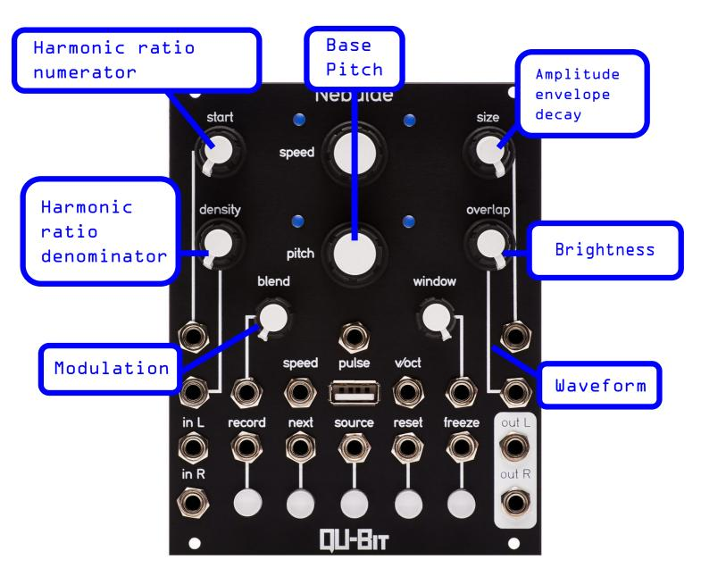
The percussion drum is a four operator phase modulation voice with operator frequencies set by an integer numerator/ denominator ratio. The 'blend' knob will increase phase modulation amount from each operator to the next, waveform crossfades between a sine wave and a tangent (similar sound to a saw tooth). Brightness controls cutoff frequency of a low pass filter.
