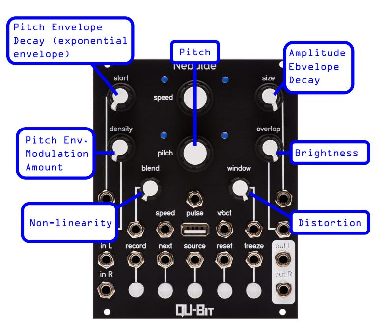
The bassdrum consists of 3 sine wave oscillators that are all ring-modulated and then sent through a low-pass filter. "Nonlinearity" controls a sort of detune for each of the oscillators as well as an overdrive of the filter.
