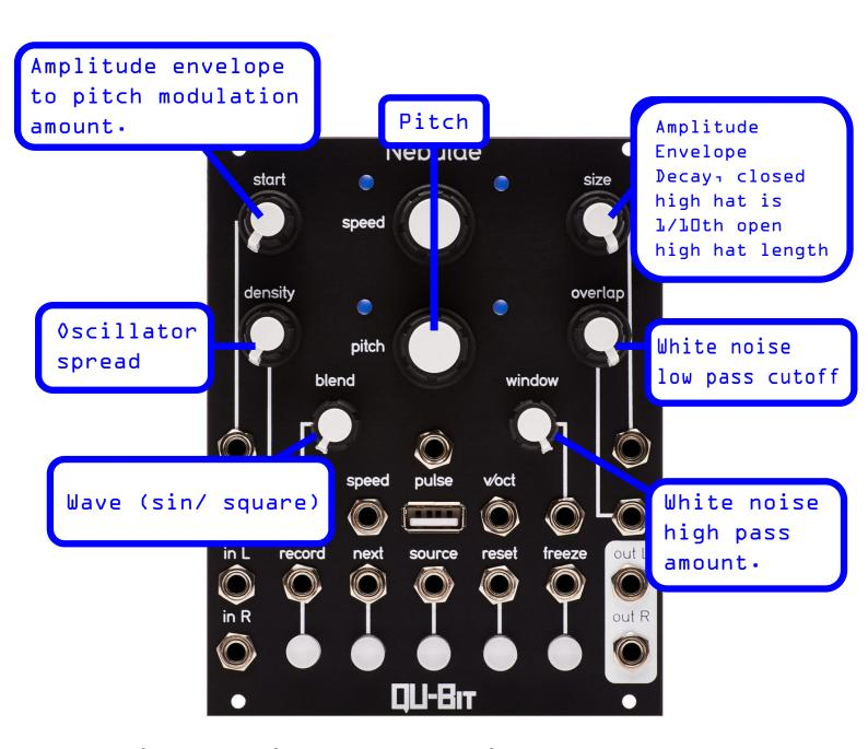
The high hat is a set of ring-modulated oscillators and white noise with both high pass and low pass controls. The closed high hat decay is a preset fraction of the length of the open high hat decay (roughly 1/10th). Window works in the opposite direction of how a high pass filter is normally configured to work nicely with the window knob response on other drums.
